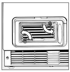
■ Turn both the levers on the condenser unit to the vertical position.
